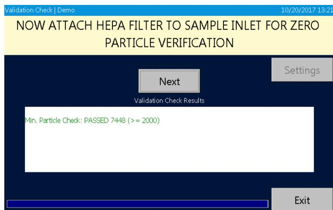
If a leak occurs in the sample train of the device, the test result may be affected. The Zero Check determines that there are no internal leaks or loose connections. Install the HEPA filter to the clear sample inlet line (making sure that the arrow on the HEPA cartridge is aligned with the flow), and tap [Next] to begin the Zero Check measurement. When the Zero Check is complete the AccuFit 9000 automatically continues to the next check.
