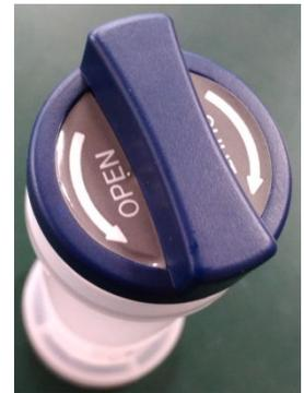
3. Pour isopropyl alcohol in the alcohol storage container up to the marked level. Be careful not to tip the bottle and spill the alcohol prior to seating the wick or storage cap, Once the wick assembly or storage cap is seated securely in the capsule the alcohol will not leak.
