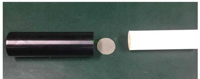
2) Remove the wick and mesh from the cartridge cylinder.
