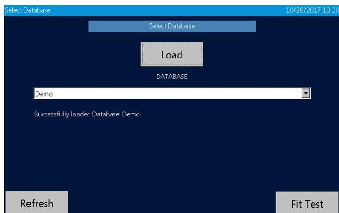
Insert the USB flash drive into a USB port Type A (H) of the device, prior to performing Validation Check (2). Select the desired database and tap [Load] then tap [Fit Test] or [Exit] button.
