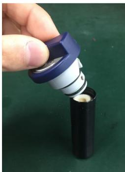
1) Disassemble the Alcohol cartridge.
