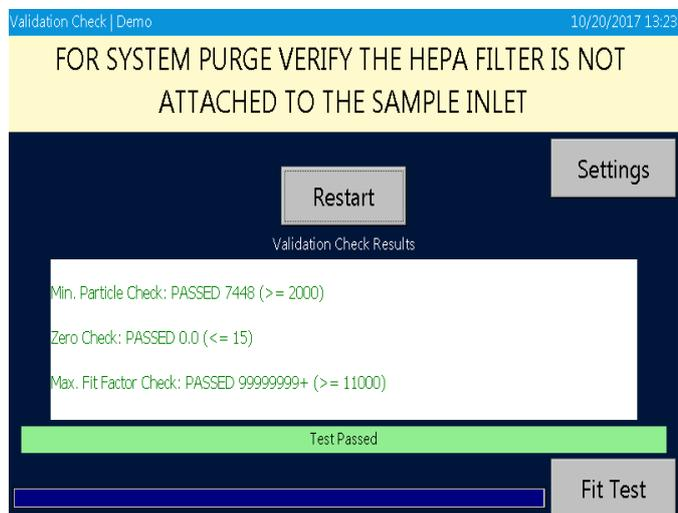
To confirm whether the device performs correctly, this test confirms the fit factor using the HEPA filter. The instrument measures the particle concentration in the ambient air and calculates the ratio to the particle concentration via the HEPA Filter. By determining this ratio, the device confirms that it is correctly performing this function.
